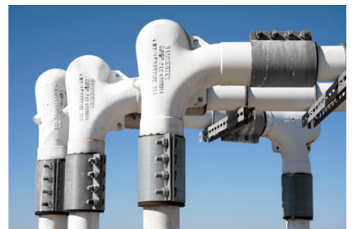
The protruding vortex chamber of the Smart Elbow® deflection elbow creates a flow path that prevents abrasive sand from impacting the elbow wall.
