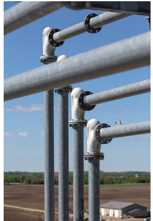
These Smart Elbow deflection elbows reduce aeration of dry cement powder moving through the pneumatic lines, decreasing dust collection demands.
